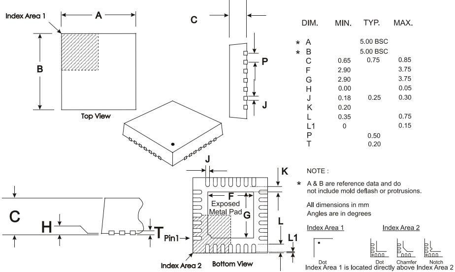
Depending on the method of lead termination at the edge of the package, pull back (L1) may be present.
